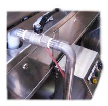
The oil load in the fryer can take automatically (controlled by the MAX and MIN levels) or manually.
