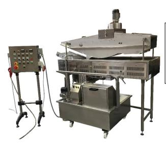
To facilitate the cleaning process, it is possible to automatically raise the cooking belt from the fryer tank, by means of two buttons placed in the control panel.
